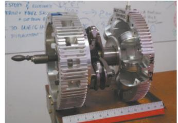
By repositioning the combustion components in a circle, the MYT engine eliminates mor e than 80 percent of all parts found in a traditional engine.
