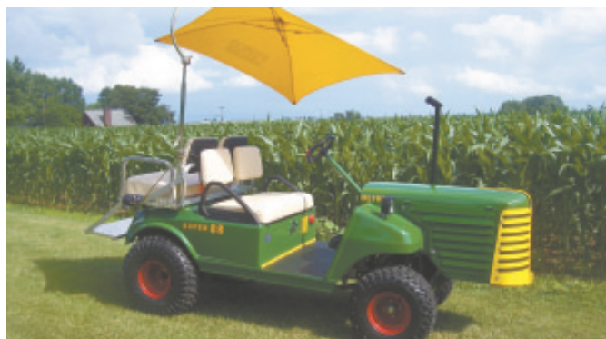
Oliver golf cart was made by cutting the front off an Oliver tractor and attaching it to a golf cart. Owner George Weyhrich and his wife enjoy driving it at farm shows.
