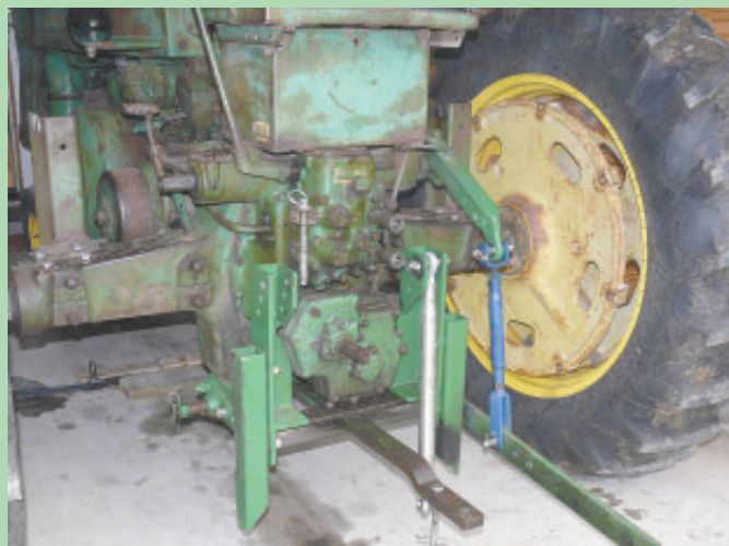
Jim Colsch built this heavy duty quad link hitch on back of his Deere 60 tractor.
