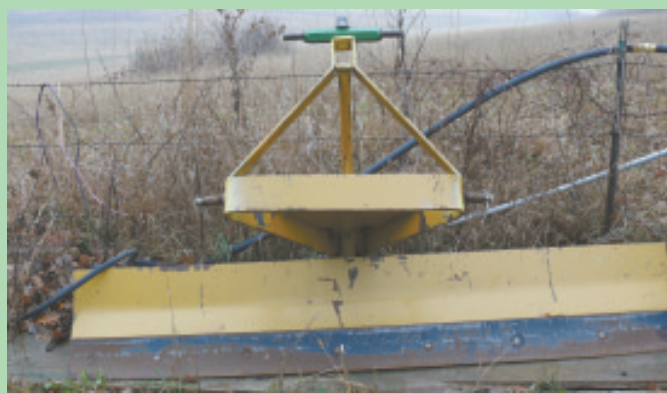
Jim Colsch built this heavy duty quad link hitch on back of his Deere 60 tractor.
