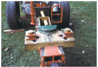
Pipe pusher is shown here ready to bend 1-in. dia. pipe. Pusher rides in a 1-in. wide groove and is moved along by a 2-in. dia. shaft that fits into log splitter's push plate.
