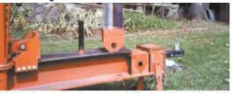
Splitting wedge sets in 6-in. wide recess in top of splitter beam. It's secured by a 1 1/2-in. dia. pin. Photo shows log splitter wedge removed and setting on top of beam.
