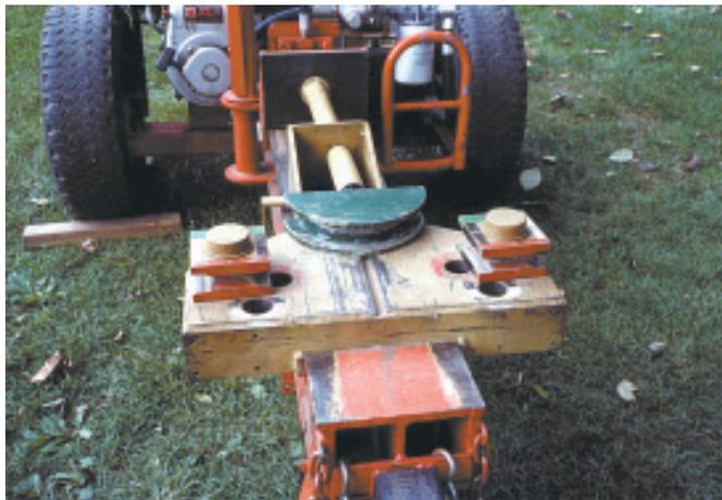
Pipe pusher is shown here ready to bend 1-in. dia. pipe. Pusher rides in a 1-in. wide groove and is moved along by a 2-in. dia. shaft that fits into log splitter's push plate.
