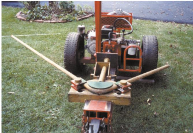
Pipe bender works like a log splitter. It consists of a semi circular pipe pusher that slides back and forth on top of a 2-ft. wide metal box.
