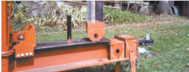
Splitting wedge sets in 6-in. wide recess in top of splitter beam. It's secured by a 1 1/2-in. dia. pin. Photo shows log splitter wedge removed and setting on top of beam.
