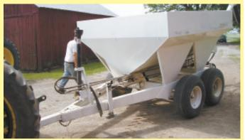
Hydraulic hoses run from tractor back to add-on orbit motor on back of buggy, which is used to drive the auger.
