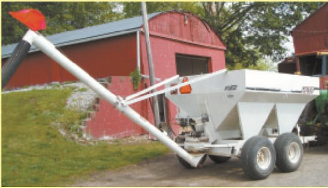
Larry Evans removed the spreader on back of a tandem axle fertilizer buggy and mounted a 6-in. dia., 12-ft. long hydraulically-powered auger.
