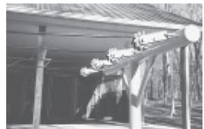
Ratchet-type electric fence tighteners are used to keep clotheslines tight.
