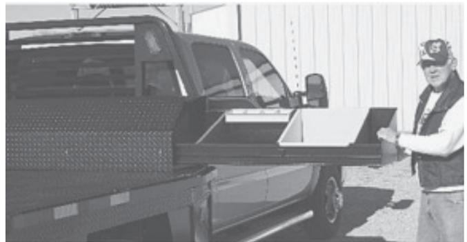
Toolbox contains a metal tray that rolls out to both sides, allowing you to get at tools from either side of pickup.
