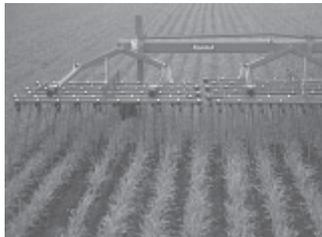
Offset tines stir every inch of the soil surface across width of implement.
