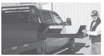
Toolbox contains a metal tray that rolls out to both sides, allowing you to get at tools from either side of pickup.
