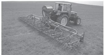
Weeder has 5 bars fitted with offset tines that kill weeds through "gentle" cultivation.
