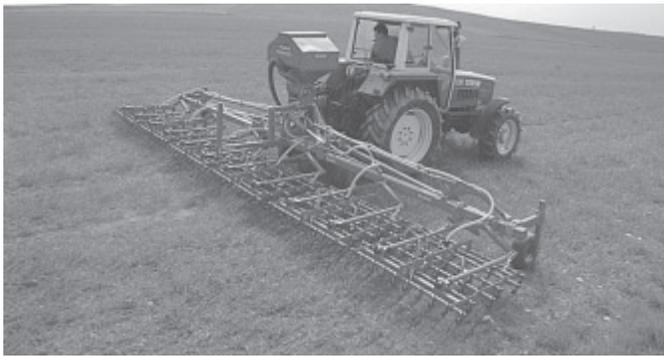
Weeder has 5 bars fitted with offset tines that kill weeds through "gentle" cultivation.
