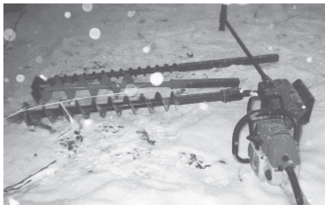
Keith Diehl converted a Stihl 041 chainsaw into a fast-working posthole digger.
