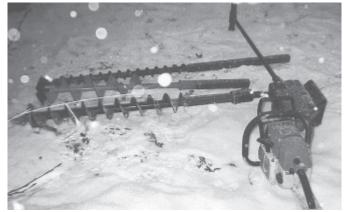
Keith Diehl converted a Stihl 041 chainsaw into a fast-working posthole digger.
