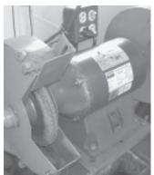
Bud Blanton stacked three chop saw wheels together and mounted them on his bench grinder. "Chop saw wheels cut at least twice as fast as grinding wheels," he
