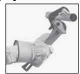
Thumb trigger is used to open or close wrench's spring-loaded jaws, which pivot on a ratchet.
