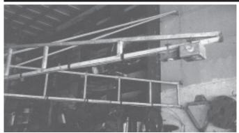
Hinged overhead boom is fitted with an electrical outlet that's always within easy reach.
