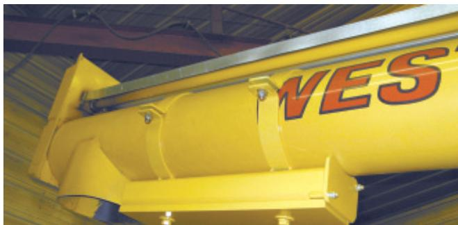
Gutschmidt added a weight box to counterbalance the lower end of his 10-in. by 36-ft. take-out auger, making it easier to lift (above). He attached a swivel caster wheel at the bottom to make the auger easier to roll around.
