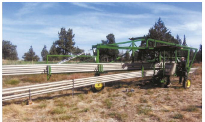
**Operator sits in a sideways-facing seat and uses a pair of remote-controlled electric winches to load and unload pipe.**
