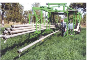
Dennis Wirt's home-built, self-propelled pipe hauler makes it easier for one person to load and unload 40-ft. lengths of 3-in. dia. irrigation pipe.
