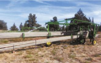
Operator sits in a sideways-facing seat and uses a pair of remote-controlled electric winches to load and unload pipe.
