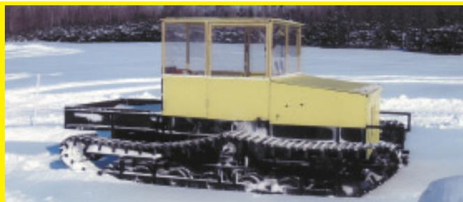
Thanks for the story on my home-built "Snow Cat" in your last issue. I thought your readers would like to see the machine in color. It's built from a 1985 Chevy Chevette 4-cyl. engine and automatic transmission connected to a Chevy S-10
