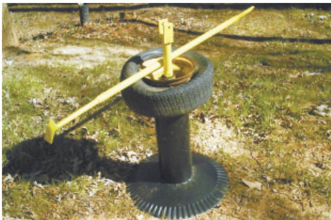
George Liskey's home-built tire changer is designed for 8-in. and smaller wheels.
