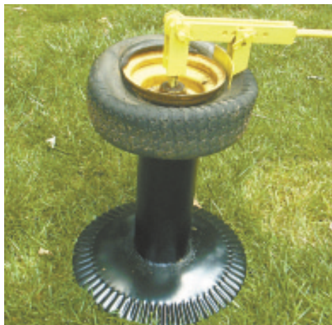
He used parts from a semi-mounted moldboard plow to build tire changer.
