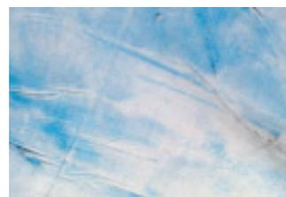
Closeup of flexible roofing material made by spreading silicone caulk on lightweight mesh fabric.
