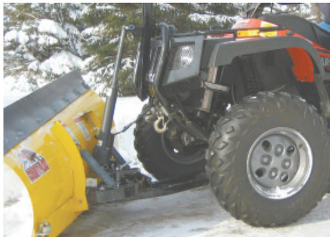
Add-on electric cylinder lets you apply down pressure to blade on ATV.
