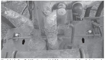
Simple latch allows Todd Quatier to use his left foot to trigger a lock on the brakes as he steps on them with his right foot.
