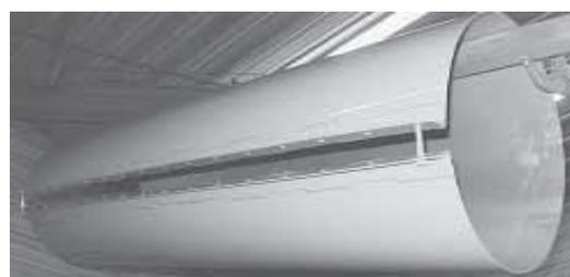
**Reinforcing sleeve fits over damaged section of unloading auger on Gutschmidt's Deere 9650 STS combine.**
