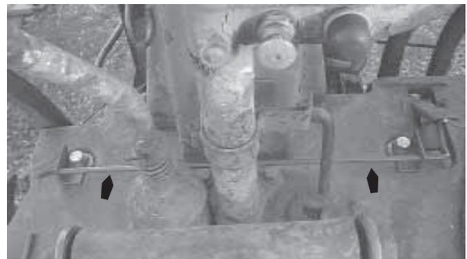
Simple latch allows Todd Quatier to use his left foot to trigger a lock on the brakes as he steps on them with his right foot.
