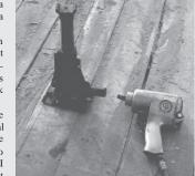
**Duwavne Bakker, Riverton, Wyoming:** Those crank jacks everyone uses take forever to raise. Here's a way to crank up a jack quickly and easily. I weld a 1/2-in. drive socket to the jack and use an electric drill to crank it up.
