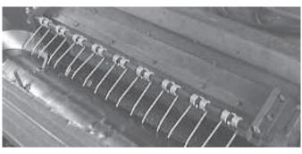
"The Buck Stops Here" attachment fits onto combine feederhouse, tearing weeds off header auger before they start to wrap.
