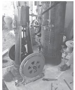
Normally, Dan Bartman uses the wind or the sun to charge up the batteries that let him live off the grid in Fort Collins, Colorado. But if he wants, he can burn wood to power a 1903 CB&H 6 hp steam engine that spins an alternator.
