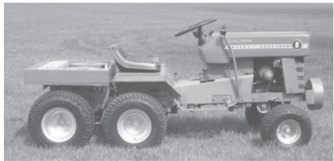
**"It lets us haul excess ground from graves dug in our cemetery without damaging the turf," says Jerry Bruecker, who converted his Massey Ferguson 8 hp garden tractor into a 4-WD, tandem axle model. He also built a high flotation dump trailer to pull behind it.**
