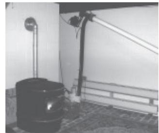
Joseph Rupinski built a large corn bin (left) in his basement that supplies his corn burning stove via an electric feed conveyor (right). Screw conveyor runs from bin to flexible plastic filler tube.
