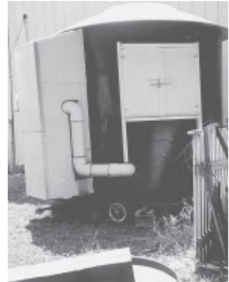
"It's big enough to hold large parts and is easy to move around," says Ron Hanen, who made his own portable sandblaster using a 3,000-gal. plastic water tank and an old satellite dish.
