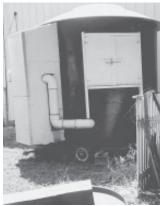
"It's big enough to hold large parts and is easy to move around," says Ron Hanen, who made his own portable sandblaster using a 3,000-gal. plastic water tank and an old satellite dish
