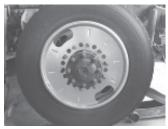
Centramatic Wheel Balancer consists of a bolt-on steel disc with a closed metal loop around the perimeter that's filled with metal nellets and fluid.
