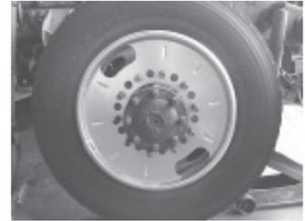
Centramatic Wheel Balancer consists of a bolt-on steel disc with a closed metal loop around the perimeter that's filled with metal pellets and fluid.
