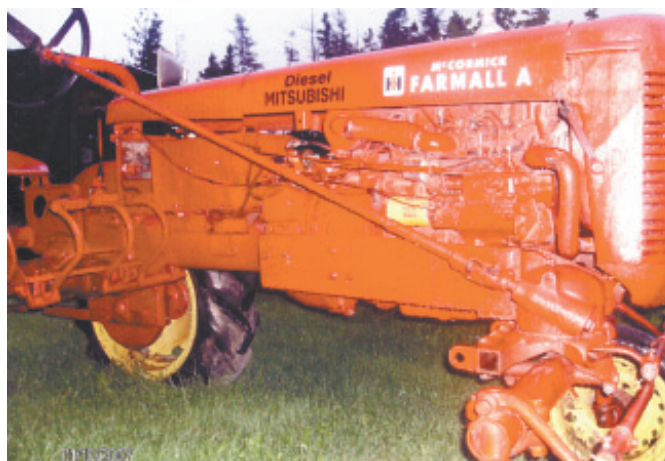
Restored Farmall A is powered by a Mitsubishi diesel stationary engine.
