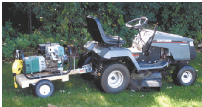
Bill Noyes uses a home-built trailer to pull his Coleman 5,000-watt generator behind his Sears riding mower. He uses it to power an electric chainsaw and hedge clippers.
