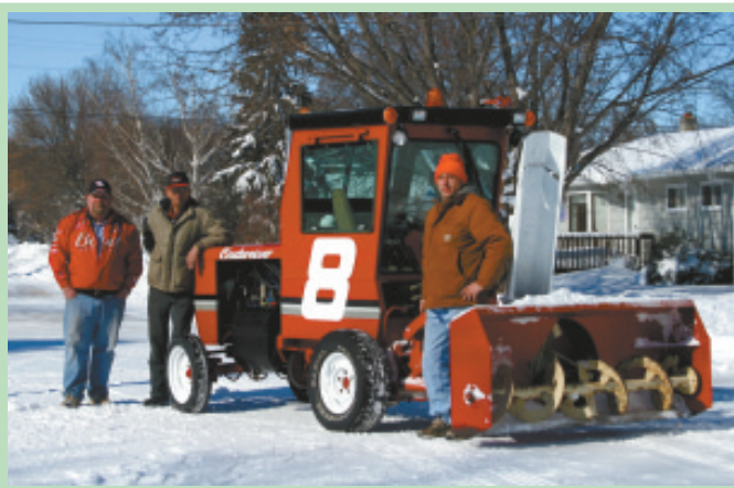
Built largely from swather components, self-propelled snowblower is painted and detailed like Dale Earnhardt Jr.'s NASCAR racer.
