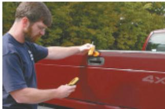
Magnetic camera is easy to position using the handheld video receiver.
