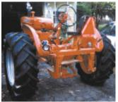
Don Kuch built this 3-pt, hitch for his Allis Chalmers WD 45 tractor. "I bought a rotary tiller for it to till my garden and a 7ft, grader blade that I use for snow," he savs.
