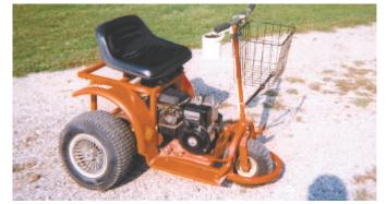
Gas-powered scooter uses parts off a rear engine riding mower and has bicycle handlbars.
