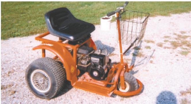
Gas-powered scooter uses parts off a rear engine riding mower and has bicycle handlebars.
