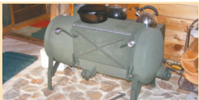
Wood burning system makes use of a 50-gal. water heater tank, with a 13-gal. heating tank added on back of it.
