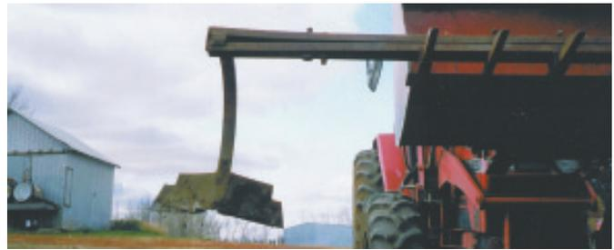
Digger consists of a cultivator shank and sweep attached to front-end loader.
