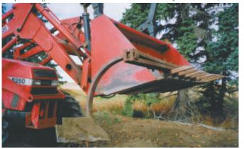
Sweep's wings have been twisted to give them a more aggressive angle. Martfeld also welded flat steel plates to sweep, widening it by an inch or two on each side.
