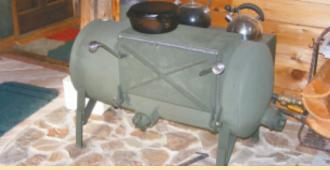
Wood burning system makes use of a 50-gal. water heater tank, with a 13-gal. heating tank added on back of it.
