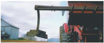
Digger consists of a cultivator shank and sweep attached to front-end loader.
