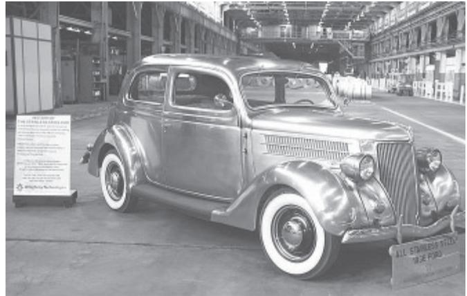
Back in 1936 Allegheny Ludlum Steel worked with Ford Motor Co. to build the world's first stainless steel car.
