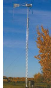
Alvin Troop put up this 5,500-watt wind turbine, called the Breezy 5.5, on a homemade 73-ft. tower.
