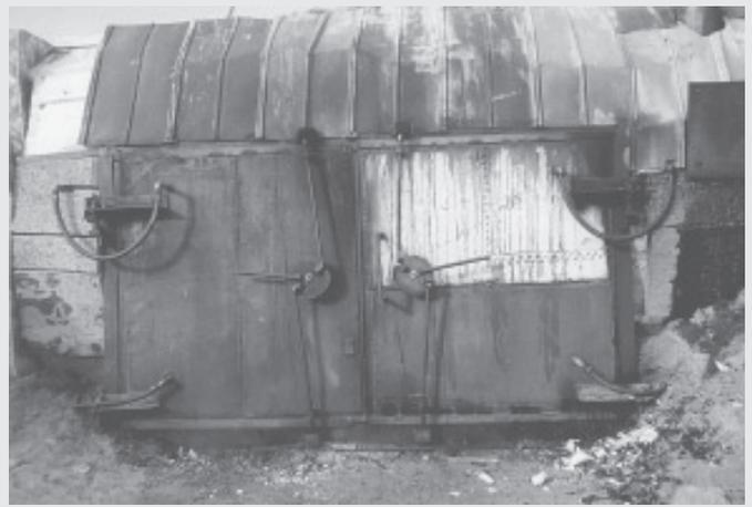
Stove is fitted with a pair of 5 1/2 by 6-ft. tall doors. The wide opening allows a Bobcat to dump a load of 8-ft. wooden slabs into stove and makes it easy to haul out ashes.
