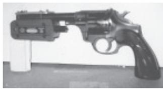
Battery-operated, carpenter's laser light straps onto gun barrel. "It projects a small red dot wherever I aim," says Ken Voigt.
