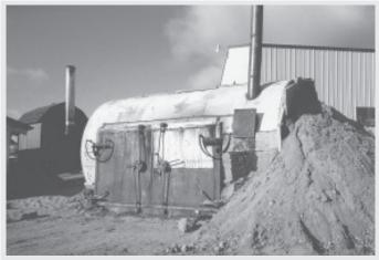
Louie Shively used a 10,000-gal. fuel tank to build this giant outdoor wood stove. Back side of stove is banked with dirt for insulation.
