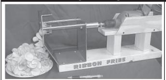
Drill-powered machine turns a potato into one long curly strip.
