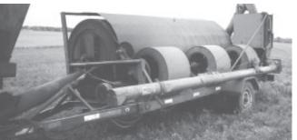
Mobile roaster keeps custom operator Ken Ressler busy all year long. Roasted grain is cooled in this drum, which is fitted with several large electric fans.
