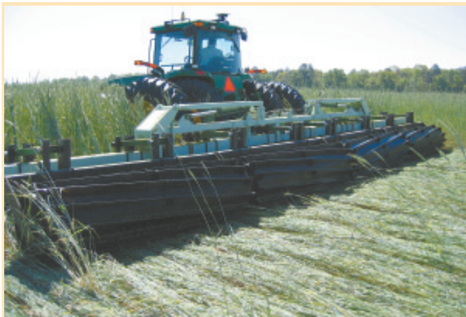
Jimmy Brooks uses his 40-ft. home-built roller to crush heavy rye cover crops.
