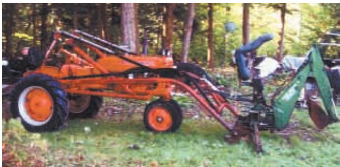
Edwin Bienvenue mounted a Deere backhoe on his Allis Chalmers C loader.
