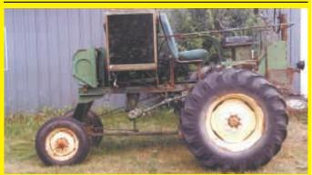
I needed an extra tractor to pull wagons to the field. I didn't want to spend the money for another tractor so I made my own by cutting down a 1953 model 55 Deere combine. I shortened the frame 4 ft. and used angle iron to reinforce the frame. It still uses the original belt drive to the transmission. I added a school bus
