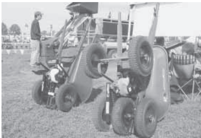
Photo shows 2-wheel-drive model, left, and 3-wheel-drive model, which is also fitted with optional rear wheel kit.
