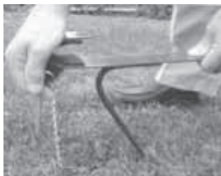
You push the "Mower Tilt" pin into the ground with your foot, hook the mower handle under the bracket, and fasten it in place with a pin.
