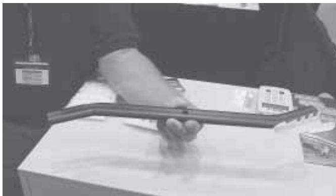
Poly cutting tips, right, slip into blade holder shown above. Notches on tips help mulch grass.
