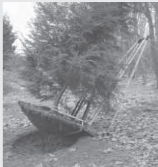
Tree lifter consists of four steel posts attached to a rectangular base.
