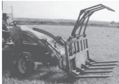
Mel Pralle built this grapple fork using the frame off an old field cultivator. “It's big enough to pick up large quantities of brush and wood, yet is lightweight enough for my New Holland 35 hp tractor,” he says.
