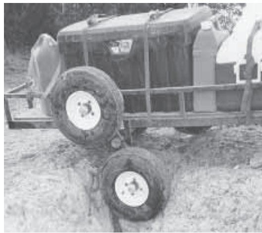
Trailer's wheels are designed to float up and down over changes in terrain, to the point they'll actually flop one wheel over the other, if necessary.
