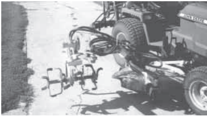
To build side-mount tiller, Houska stripped an old tiller down to the tines and fitted it with a belt-driven hydraulic motor. It connects to two hydraulic cylinders on tractor.
