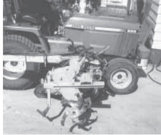
One cylinder moves tiller in and out; the other tilts the tiller sideways.
