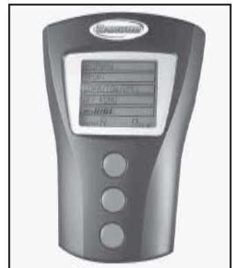
Remote-controller activates an air compressor that lets you select the firmness of the ride.
