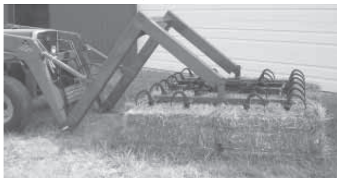
Home-built, loader-mounted bale clamp is used to move bales into barn. It grabs 12 bales at a time and can stack them up to 14 ft. high.
