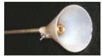
The 4-in. dia. cone is made from heavy duty plastic and is held on by a couple of screws.
