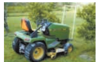
"Cobweb catcher" is made from 3/4-in. dia. plastic pipe. It mounts on a steel frame welded onto front of mower.
