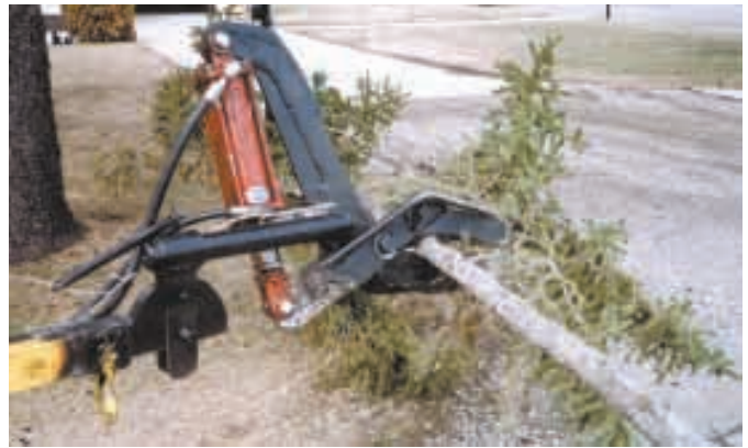
Shears operate off a 2 1/2-in. hydraulic cylinder that opens up to 8 in.
