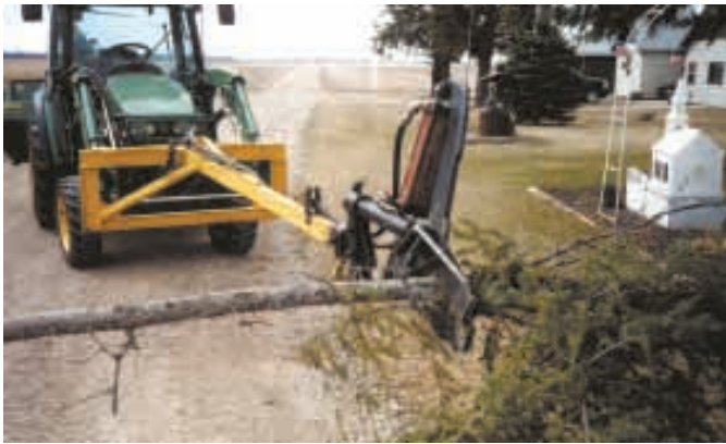
Tom Houska's home-built hydraulic tree shears mounts on a boom he made for his tractor loader.
